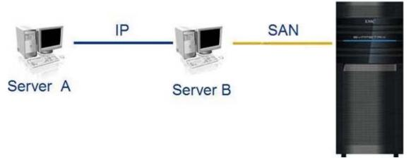
Symmetrix Management Console will be deployed in a remote configuration on Server A. Server A can access Server B over an IP network. Server B has access to the Symmetrix array over the SAN. Which license(s) is required on Server A?
