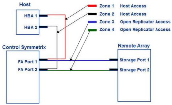
Which Open Replicator operations can be performed between the Symmetrix V-Max array and a third-party array based on the architecture shown in the exhibit?
